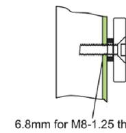
Inside: Drill a hole diameter is 8mm folding the plastic straightpin
